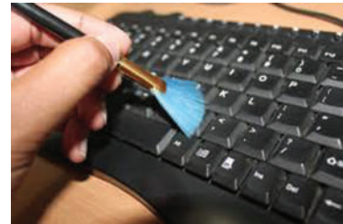
Figure 3.21: Cleaning keyboard with soft brush
